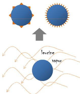
**Figure 2.** Continuous aerosol process to produce fine powders with a leucine coating of tunable roughness.
